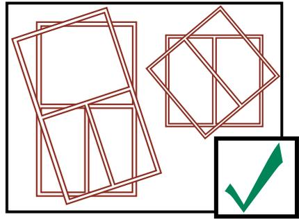
Do not lean windows against a tree or post as they can be subject to permanent damage until installed into the building envelope. If the site is bare, lay frames flat on top of each other with weight evenly distributed to avoid buckling and distortion.
