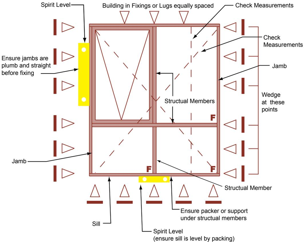
\* Fix via building lugs, nails or shim at equally spaced arrow points.
